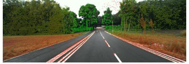
Figure 8: Illustrative LiDAR 3D point cloud overlay onto the right stereo image (colour) using the calibration obtained.
