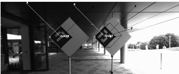
Figure 7: Camera to LiDAR custom calibration pattern with extrinsic parameter estimation overlay shown.
