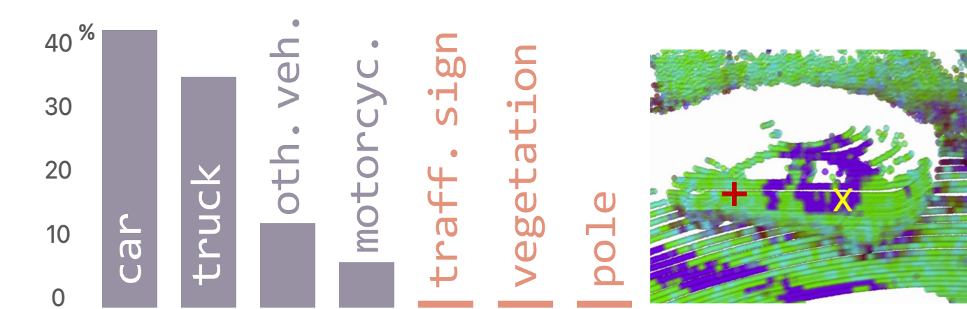
UPL Figure 3. Illustration on Unreliable Pseudo-Labels (UPL). Left: entropy predicted from an unlabeled point cloud – greener: lower entropy. Right: Category-wise probability of an unreliable prediction.
